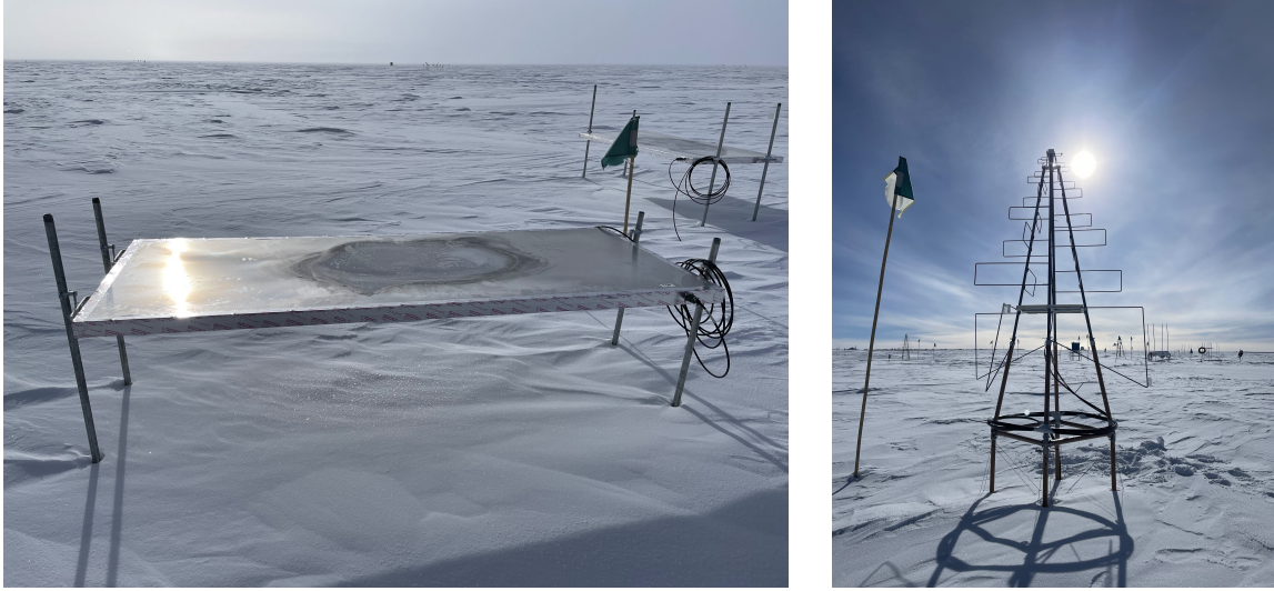
Figure 3: Photos of the detectors of the prototype station that were deployed in January 2020 taken almost three years later in December 2022. Left: One of the four pairs of scintillation panels. Right: One of the three SKALA v2 radio antennas. The concept of elevating the detectors successfully avoids snow accumulation above the detectors and enables to easily raise them every few years corresponding to the rising snow level at the South Pole. Photos courtesy of Roxanne Turcotte.
