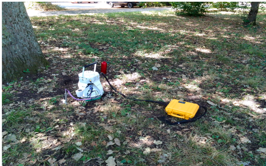
Fig. 2. The complete soil respiration field survey setup. A yellow LI-870 CO 2 /H 2 O Analyzer is next to the white Smart Chamber, sitting on the green PVC soil collar. The Stephens HydraProbe is installed adjacent to the soil gas chamber in the ground to measure soil temperature and soil water content. (Photo: Somidh Saha).
