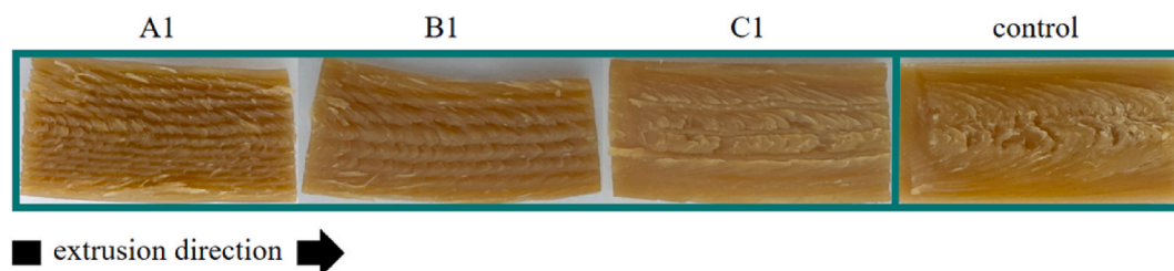
Fig. 8. Torn-open extrudates from extrusion with breaker plate of varied hole diameter (A1 = 1 mm; B1 = 1.5 mm; C1 = 2 mm) and a control extruded without breaker plate. All extrudates are oriented in the extrusion direction left to right with an extrudate width of 19 mm.
