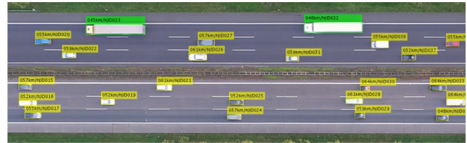
Fig. 1: Our evaluation is based on the highD dataset and predicts car-following model parameters in highway driving scenarios [7].
