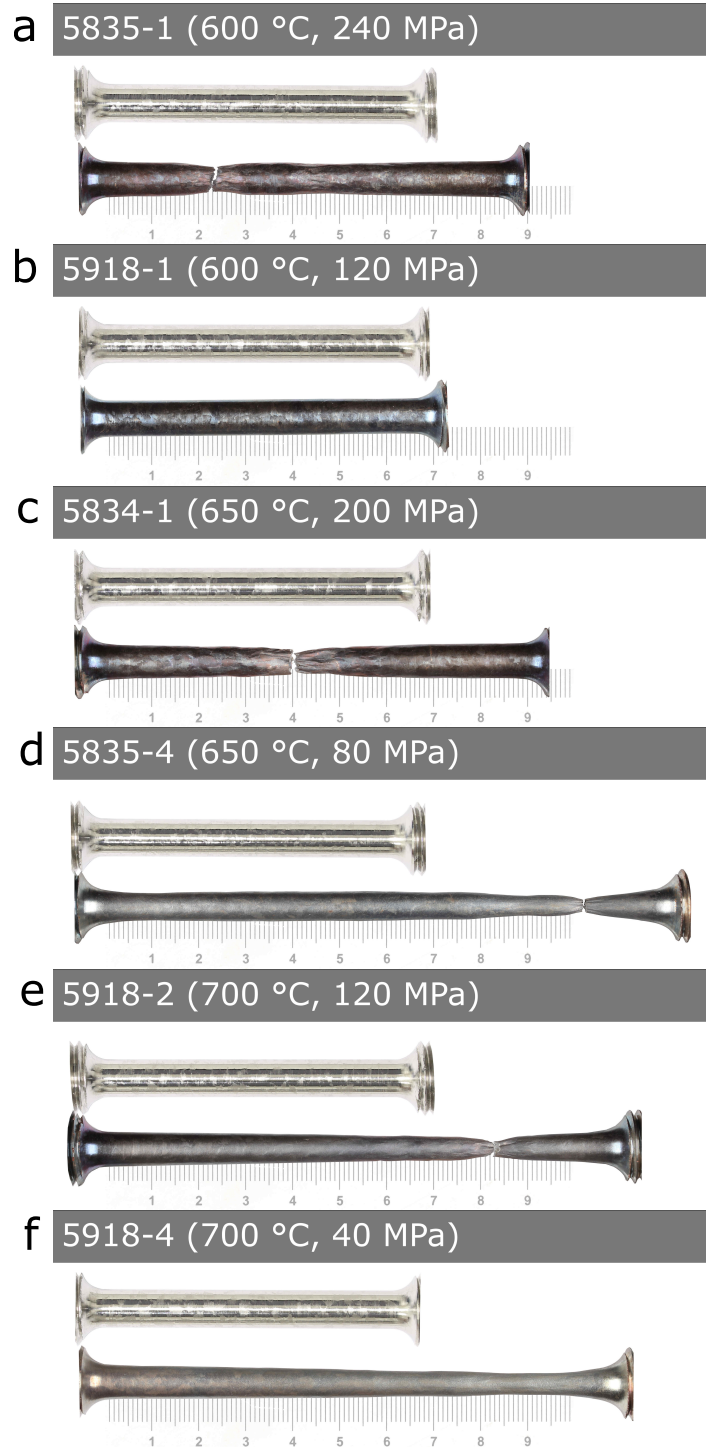
Figure B.3.: Comparison of the creep specimen geometry before and after the creep test of Fe-25Al-3.7Mo-0.4Ti-1B [143]. The images compare the maximum and minimum stress levels tested at the three test temperatures 600 °C (a,b), 650 °C (c,d) and 700 °C (e,f).
