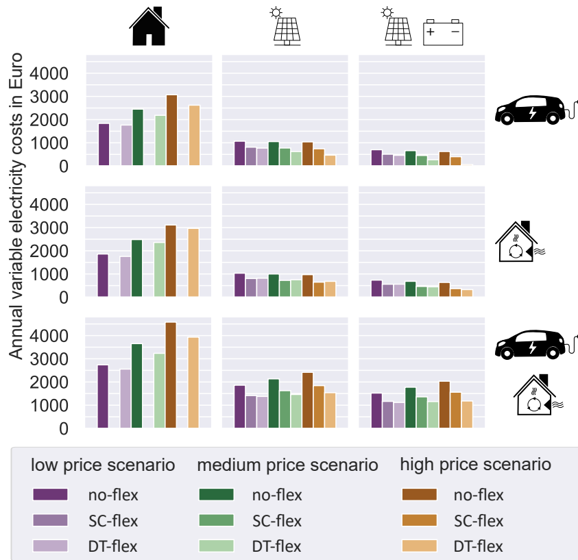
Figure 7.7: Annual variable electricity costs (unit rate costs minus feed-in remuneration) for the no-flex, SC-flex, and DT-flex cases for all three price scenarios (average over all households).
