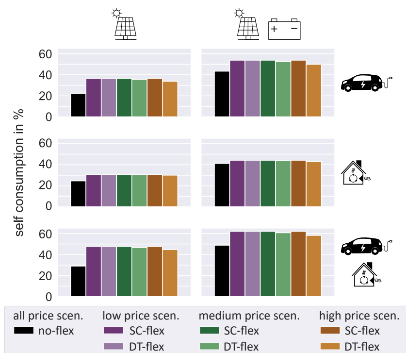
Figure 7.6: Average self-consumption rate for the SC-flex and DT-flex case for all three price scenarios.
