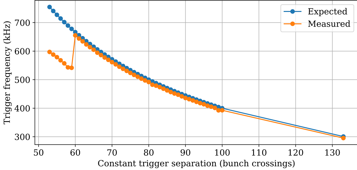
Figure 6.17.: Expected and measured trigger frequencies over the CTS value. The measured trigger frequency is always lower than the expectation since some triggers fall into the orbit gap and get rejected. The drop at a CTS value of 59 bunch crossings is caused by the CMS trigger rules (see table 6.3). Rule 4 becomes relevant as soon as the CTS value is below 60 bunch crossings.
