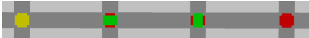
Figure 3.22: The four statuses of conflict areas in PTV VISSIM. From left to right: passive, two-yields-one, one-yields-two and undetermined.
