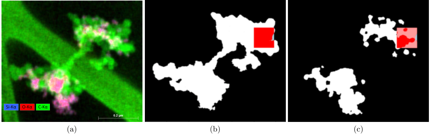
Figure 2: Workflow of image processing. (a) Unedited EDX scan of a hetero-aggregate. Segmented image of the carbon structure (b) and the silica structure (c) within the hetero-aggregate with evaluated image cutout. In the evaluated image cutout in (c), the silicon content is marked with dark red, the carbon content within the image cutout in mute red and the background in blue.
