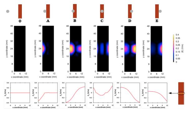
Voltage generation occurs only in the area of the tape where magnet traverses.
