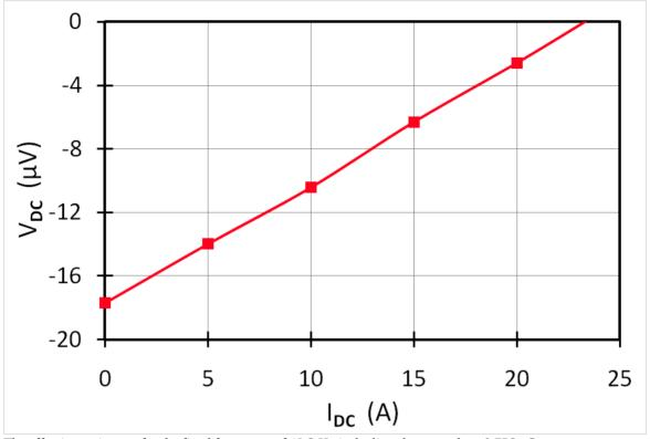
The effective resistance for the fixed frequency of 12.3 Hz is the line slope equal to -0.756  $\mu\Omega$ .
