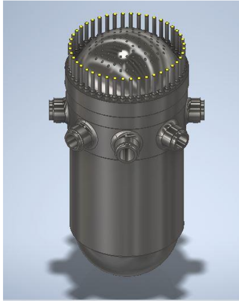
Figure 3. CAD render of the Reactor Pressure Vessel design created using Autodesk Inventor.
