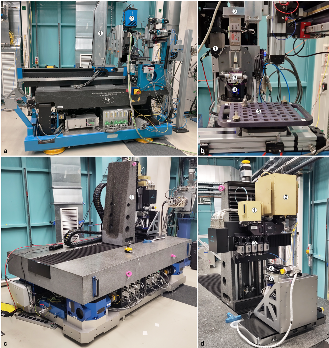
Figure 8 (a) UFO-I station for high throughput tomography in Experimental Hutch 2: (1) motorized detector tower, (2) pco.dimax camera. (b) Detail of the UFO-I sample exchanger with a tray for 49 samples: (1) white beam microscope, (2) sample changer gripper, (3) sample x-y linear stages, (4) rotary stage, (5) sample tray. (c) UFO-II during commissioning in Experimental Hutch 2: (1) detector tower. (d) Detail of the UFO-II quintuple magnification microscope and sample manipulator: (1) radiation shielded pco.edge5.5 camera, (2) radiation shielded Phantom v2640 camera, (3) visible light microscope with five different magnifications and camera branch selector, (4) sample x-y linear stage, (5) rotary stage.
