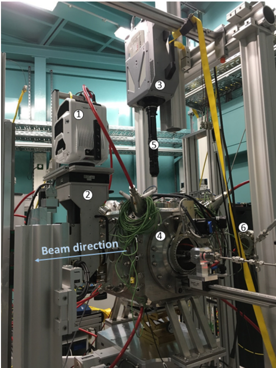
Figure 7 Custom set-up used in Experimental hut 1 for operando tomography of injection sprays: (1) Phantom v2640 camera, (2) macroscope, (3) Photron Fastcam SA-Z camera, (4) injection chamber, (5) Navitar long-distance microscope objective, (6) beam exit.
