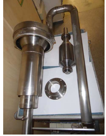
Fig. 4. Photograph of the assembled pump (left) and its components (right).
