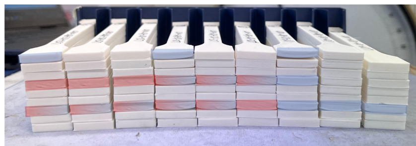
Figure 2. Side view of all samples, highlighting extrusion defects on specimens using N01 (non-rectangular outer contour/curvature (blue) and irregularities in the print image (red)).
