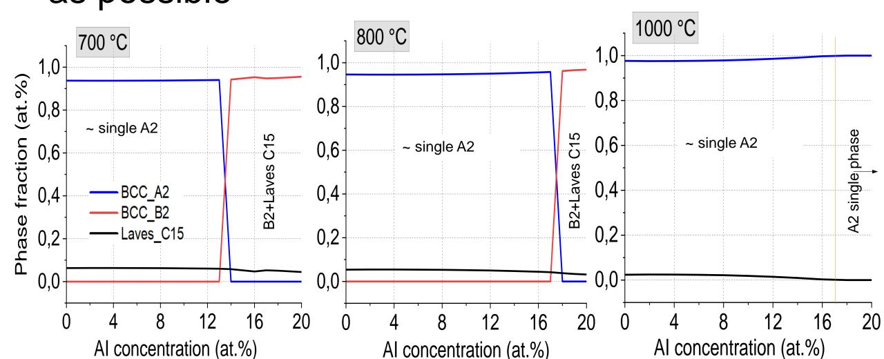
Thermodynamic modeling of the substrate yields the chemical composition 16Ta-33Mo-33Ti-5Cr-13Al (at.%). Next steps: Manufacturing and experimental validation.
