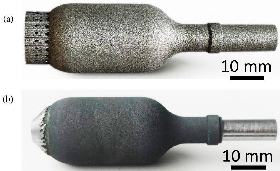
12 13 Fig. 7. Burst capsules of SLM-EF in the (a) as-printed state and (b) after HIP, heat treatment, and 14 partial lathe processing
