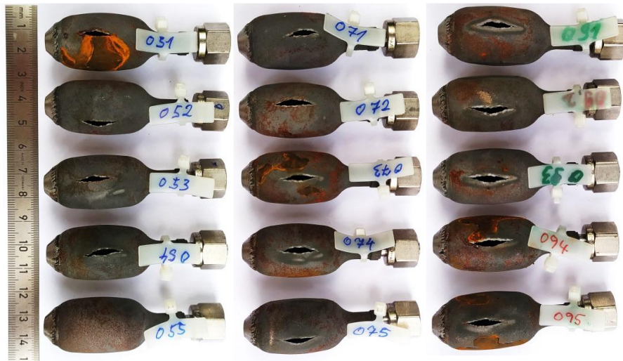
Fig. 10. Appearance of SLM-EF capsules after water burst testing. The left row has a nominal wall thickness of 0.5 mm, the middle 0.7 mm, and the right 0.9 mm.
