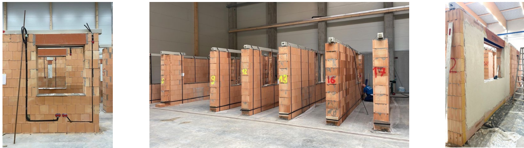
Figure 2: Impressions of the prefabrication of brick walls at the industry partner
