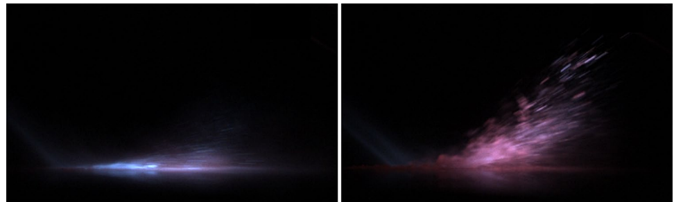
Fig. 7 Presentation of the influence of the oil temperature, 293 K (left) and 363 K (right), with an oil film thickness of 80 \mu\text{m} on secondary droplets on a smooth aluminium plate
