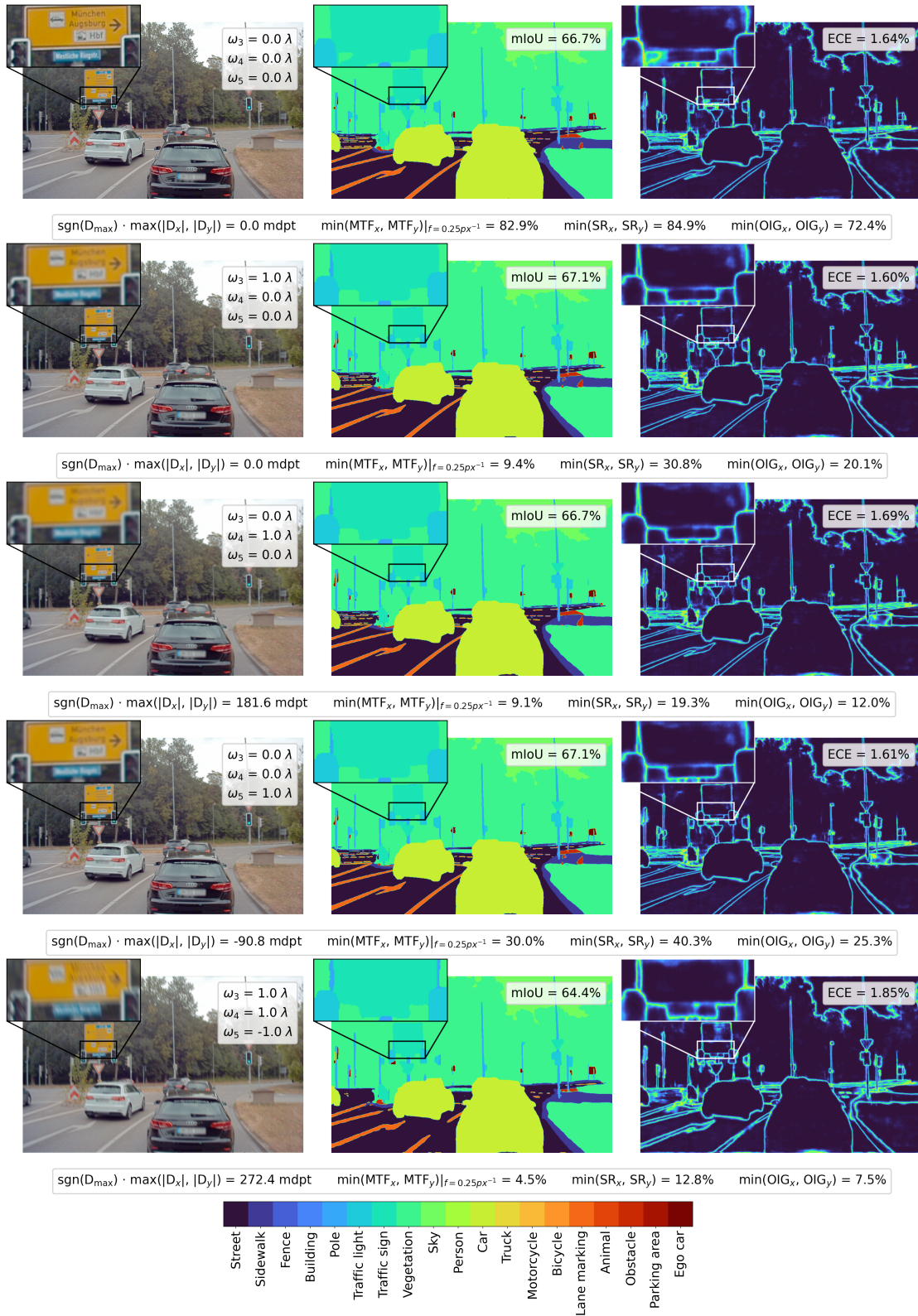
Figure 5.2: On the left, the degradation induced by the optical threat model (see Section 2.1.2) is visualized for a random instance of the A2D2 dataset for different Zernike vector parameterizations. In the middle, the semantic segmentation maps obtained by employing a customized UNET (see Section 6.2) are shown. On the right, the predictive uncertainty is visualized for every pixel based on the variation ratio. For each perturbation scenario, the optical system measures are indicated in the legend.
