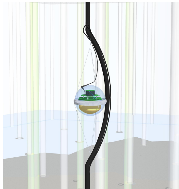
Figure 2.4.: A schematic view of an in-ice DOM.
