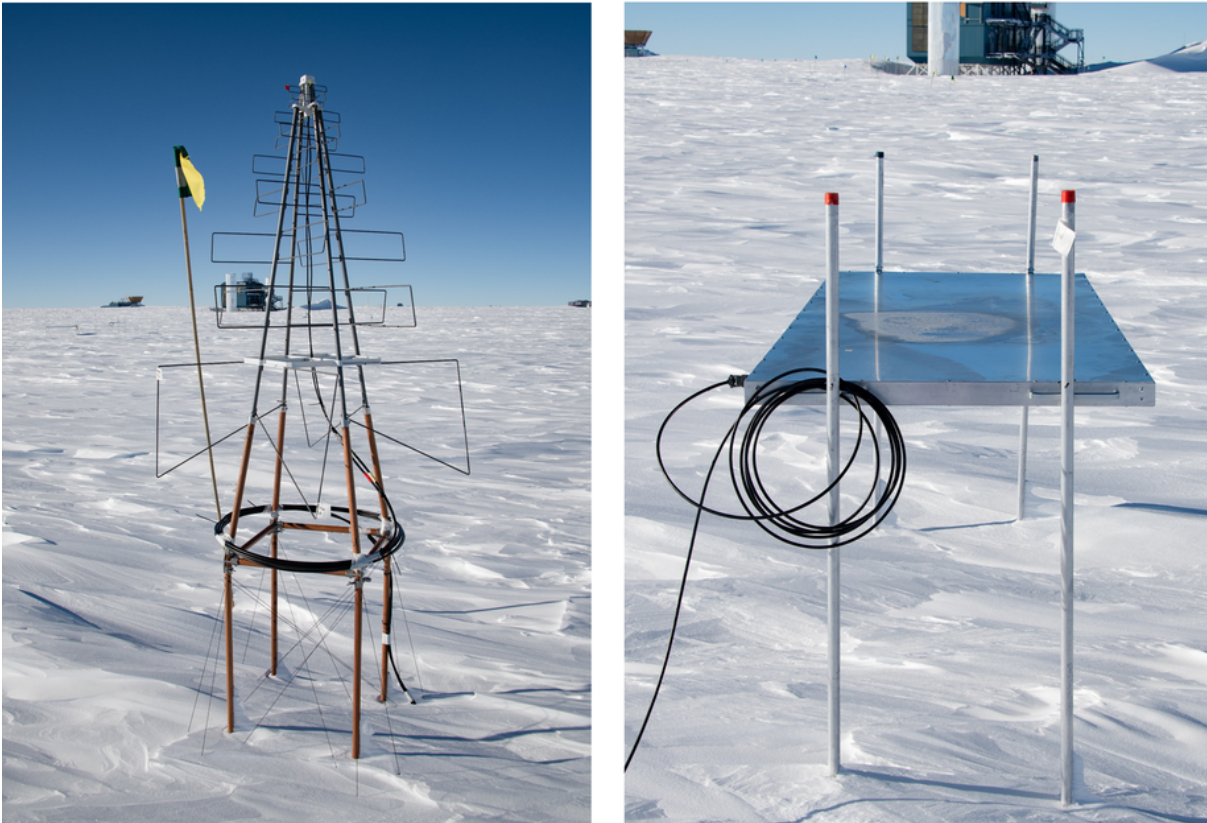
Figure 2.10.: Photos taken at the South Pole of an antenna and a scintillator panel [63].
