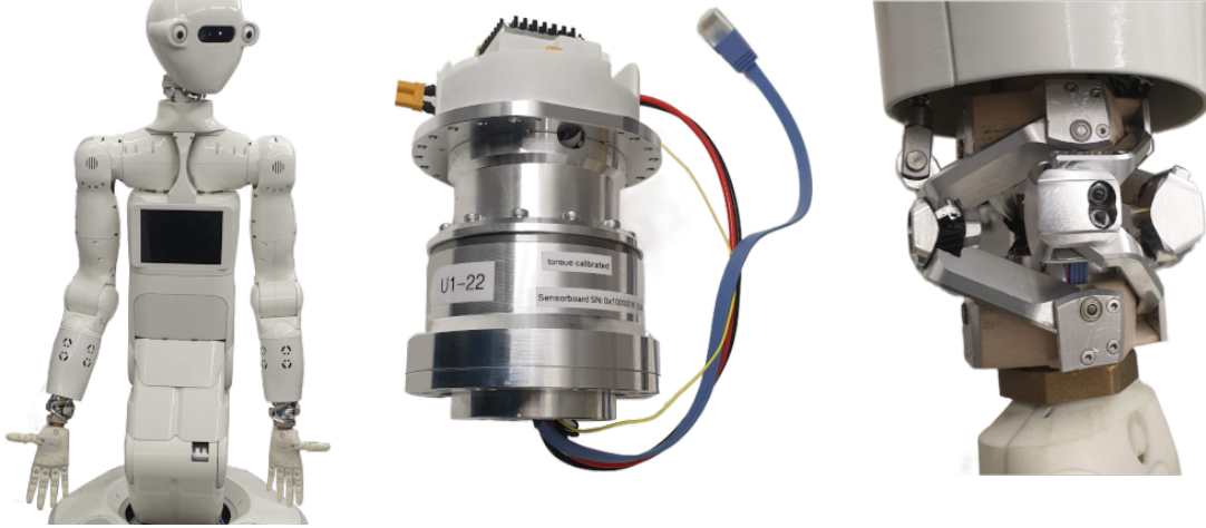
Figure 1.3.: The humanoid robot ARMAR-7 (left) and relevant arm system components: SAC units for robot joints (middle) and wrist joint mechanism (right).
