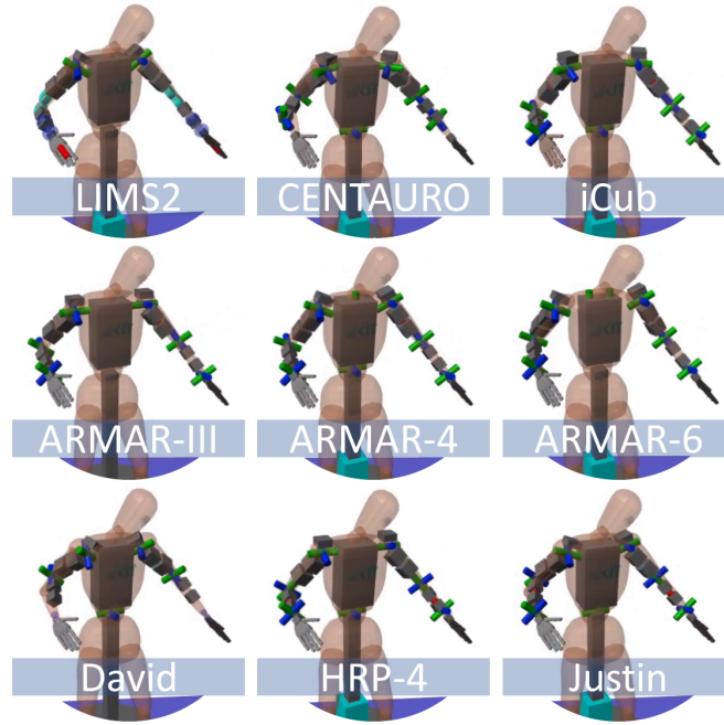
Figure 3.7.: Rendering of a unified representation of 9 humanoid robots with different kinematics performing a retargeted Conversation motion. Source: (Klas et al., 2023) © 2023 IEEE
