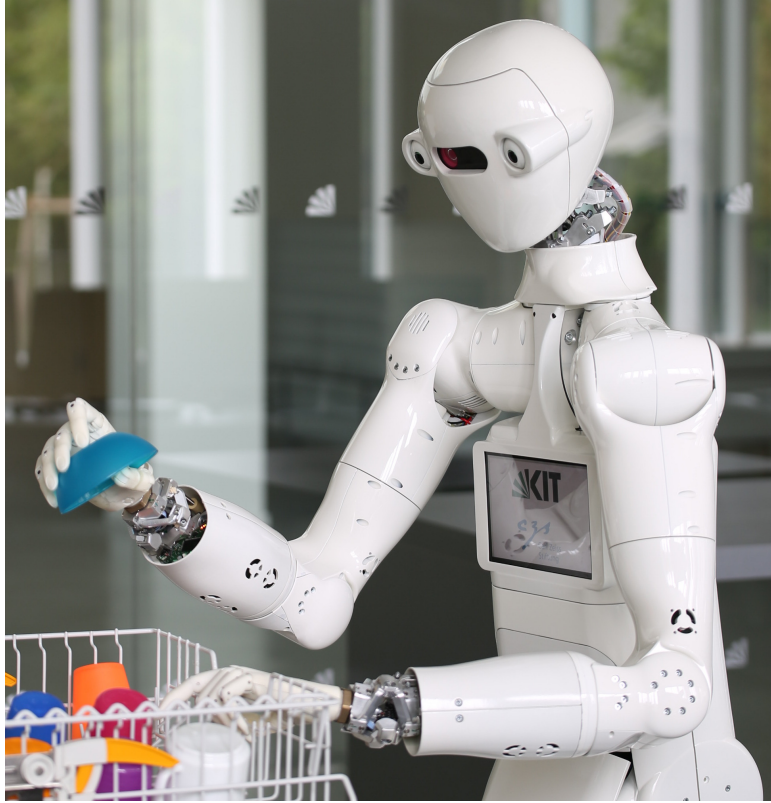
Figure 5.9.: Realization of the Quaternion Joint mechanism for the wrist and neck joints in the ARMAR-7 robot.
