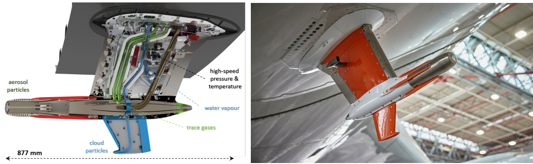
Figure 2.3: Left: CAD model of the CARIBIC 3.0 inlet system with flight direction towards the left. The inlets for water analysis are shown in blue: the total water inlet (including the collection of cloud particles) is oriented towards the front, whereas the water vapor inlet is oriented sideways. Right: Real version of the inlet system installed on the A350 during a test flight. Credits to Simon Heger and LH Technik.
