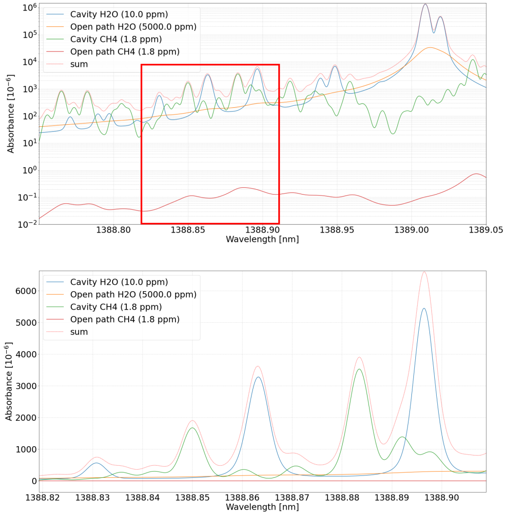
Figure 4.15: Hitran simulation of the absorption due to water and methane molecules in the open light path, i.e., at 800 mbar (orange and red lines) and due to water and methane molecules in the cavity, i.e., at 50 mbar (blue and green lines). The sum of all lines is shown as dashed red line. Nitrogen ( \sim 80\% ) and Oxygen ( \sim 20\% ) were also included in the simulation, but were not plotted because they don't show any strong absorption lines in this spectral window. Note that we did not plot the absorption per cm on the y-axis, but the absorption multiplied by the optical path length (40 cm and 30 km, respectively). The bottom figure shows a zoom into our fitting area.
