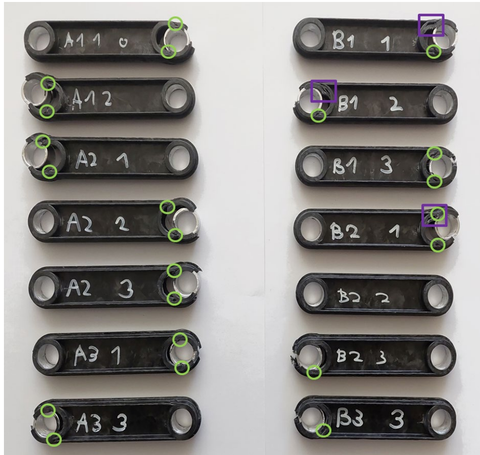
Figure 7 – All 14 test components after testing, marked with their component numbers (white), position of fracture at debonding between insert and C-SMC (green) and between rolled and flowed C-SMC (purple).
