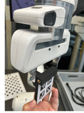
(b) Used calibration target with ArUco markers. The target can be screwed into the robotic gripper to have a fixed transformation {}^{EE}\mathbf{T}_{Target}
