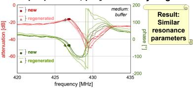
Summary: SAW biosensor devices with new and regenerated structures show the same performance in terms of physical properties.
