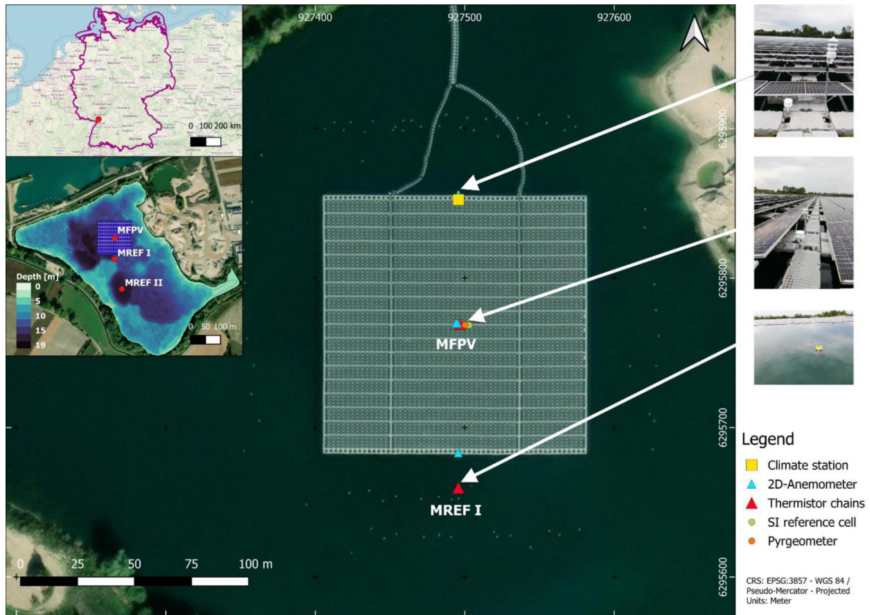
Fig. 1. The monitored floating photovoltaics (FPV) system. The two insets show the location of the studied gravel pit lake in Germany and the measurement points (MFPV, MREF I, MREF II) in the lake. The yellow square indicates the position of the meteorological measuring system.
