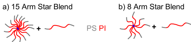
Figure 1. The blends investigated herein are made of a) triblock and 15-arm star and b) triblock and 8-arm star.
