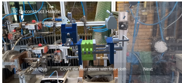
Figure 3. Integration of augmented reality (AR) with the digital twin (DT) framework [31]. This figure shows a virtual 3D model of a chamber filter press overlaid onto its physical counterpart using AR. At the current stage, the AR system primarily supports visualization of the geometry and structure of the filter press. It can assist operators by highlighting specific components—such as individual filter chambers—and providing interactive maintenance instructions, for example, indicating how to access or remove parts. This lays the foundation for future functionality, such as real-time diagnostics or condition monitoring.
