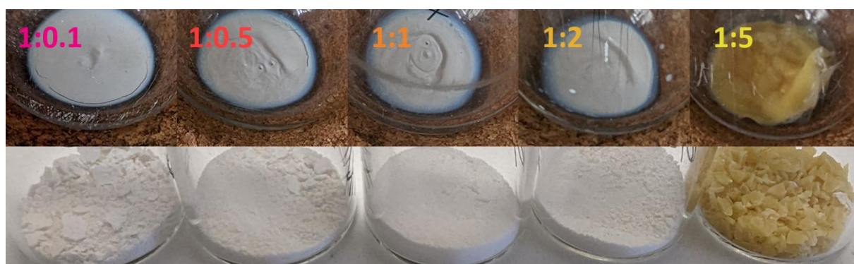
Figure 64 Pictures from PAN@SiO 2 after centrifugation (top) and after grinding in a mortar (bottom): Left to right: 1:0.1, 1:0.5, 1:1, 1:2, and 1:5 SH@SiO 2 particle mass to monomer mass ratio. All samples except 1:5 PAN@SiO 2 are off-white powders after grinding the crude particles in a mortar. 1:5 contains more PAN because assumably the high concentration of acrylonitrile triggered the Trommsdorff-Norrish-effect increasing the reaction rate significantly.
