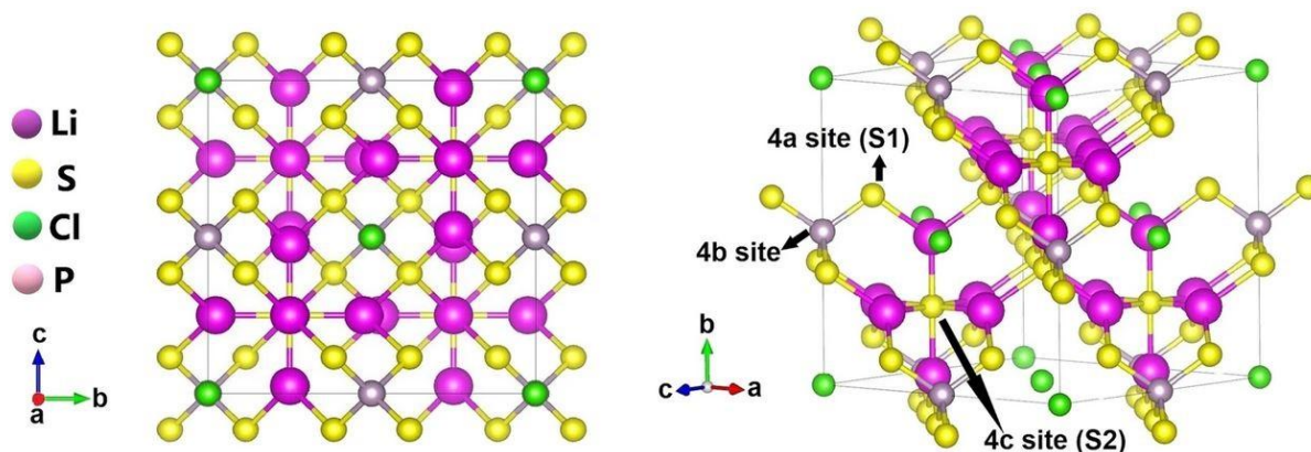
Scheme 20 Crystal structure of \text{Li}_6\text{PS}_5\text{Cl} . Reproduced from Baktash et al. with permission from Springer Nature. 261
