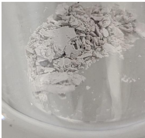
Figure 17 Picture of P7+LiTFSI coated \text{Li}_{5.5}\text{PS}_{4.5}\text{Cl}_{1.5} after drying in a vacuum oven.
