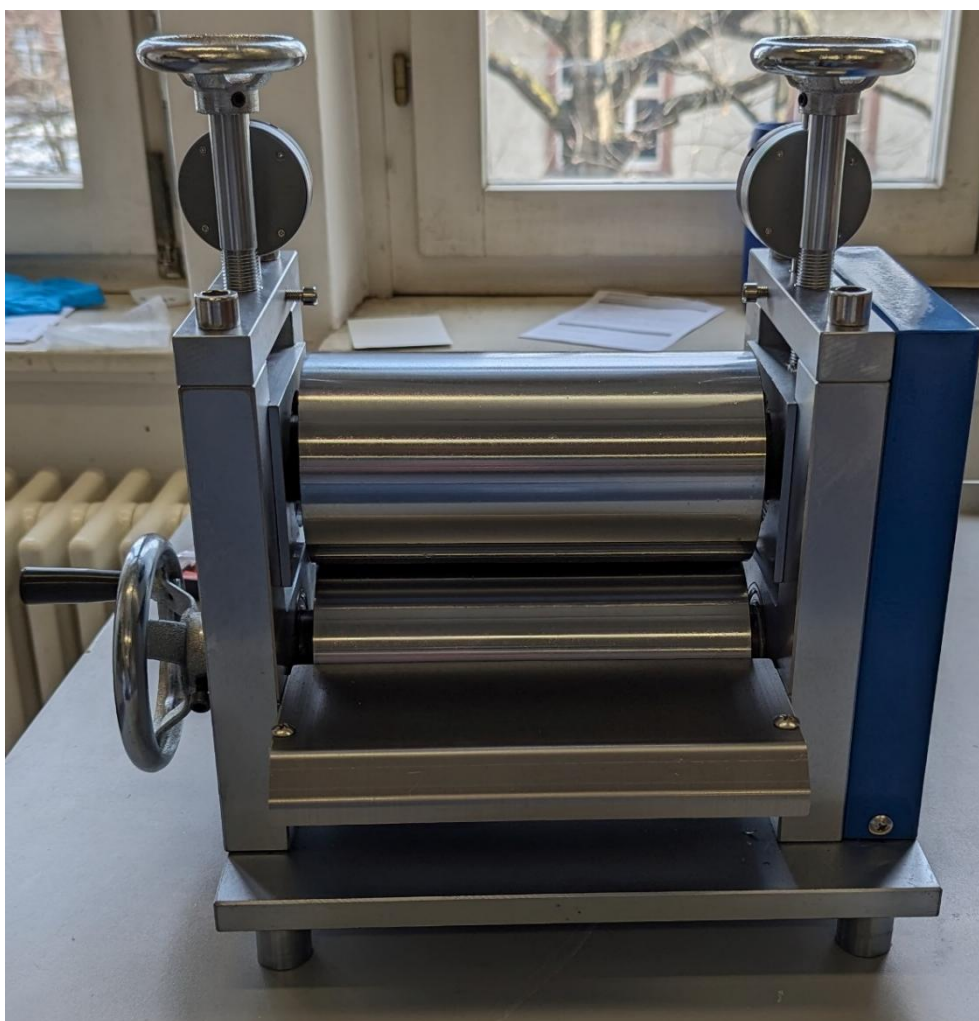
Figure 130 Picture of the manual roll-to-roll press with adjustable slit width.
