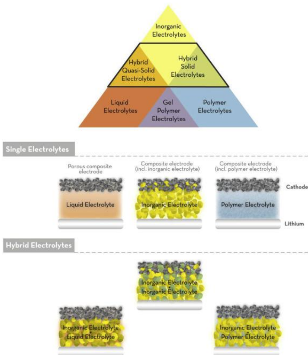
Scheme 21 Classification of hybrid electrolytes. Oxides and sulfides are combined as inorganic electrolytes. Reprinted from Passerini et al. with permission from Elsevier. 273
