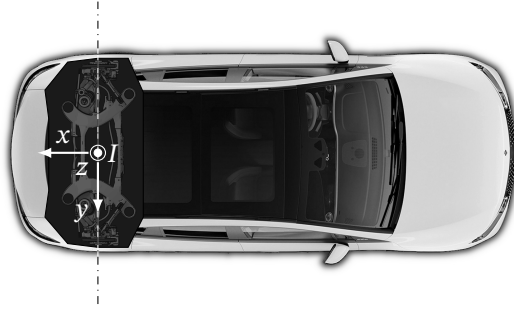
Figure 4.3: Cartesian coordinate system I for the rear suspension. The origin is located on the center of the dashed connection line between left and right wheel center point. Vehicle image part of [Mer22d].
