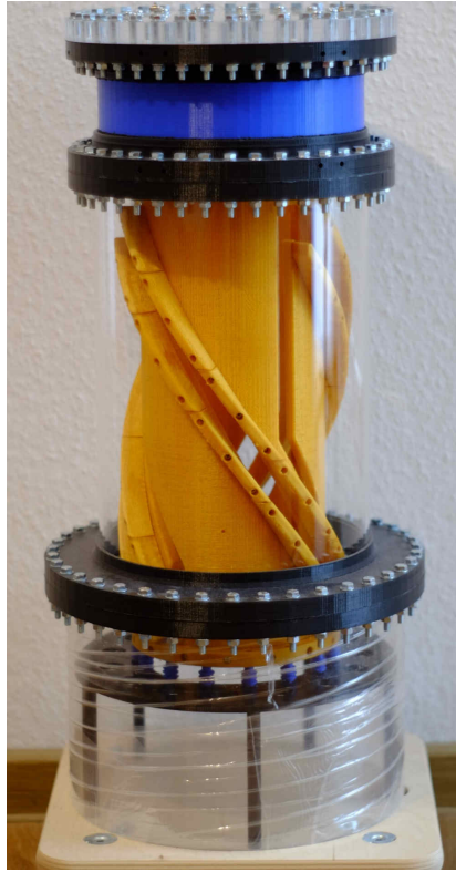
Figure 3.17: 3D printed model of the prototype for verification of assembly.
