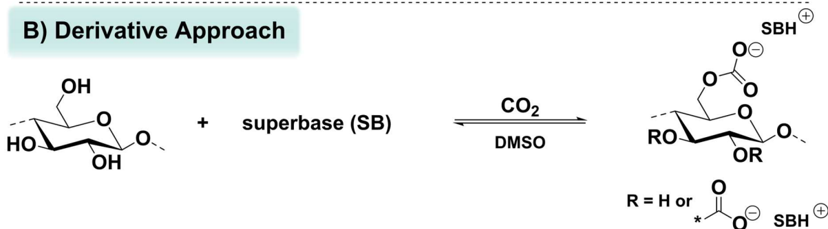
Scheme 11. General concepts for the non-derivative (A) and derivative approach (B) of the switchable solvent system for cellulose dissolution.
