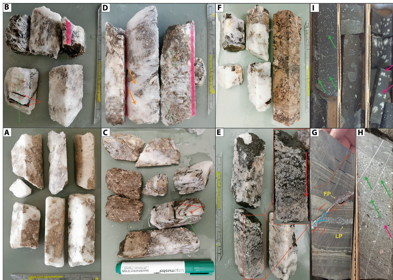
FIGURE 9 Samples with boron minerals. (A) Ibar-1, IBM2_209_210.6 m, colemanite within brecciated oil shale/microbiolites, FA9. (B) Ibar-2, IBM2_210.6_211.3 m, tabular colemanite impregnated into oil shale and dark claystone. Green arrows show mineral growth zones and red arrows show mud matrix. (C) Ibar-3, IBM2_211.1_212.1 m, tabular colemanite within brecciated oil shale, FA9. Red arrows mark mineral growth, while green trapped mudstones. (D) Ibar-4, IBM2_212.6_213.0 m, colemanite within brecciated oil shale, FA9. Green arrows mark radially oriented columnar to needle-like colemanite. Orange arrows show tabular colemanite. (E) Ibar-5, IBM6_140.7–141.2 m, colemanite crystals within dark claystone. The red arrow shows fining upwards in colemanite crystal size. (F) Ibar-6, IBM12_428.2_429.1 m, colemanite in brecciated recrystallised and brecciated microbiolites and oil shale, FA9. (G) Prodelta facie association, FA6 cross-cut by the normal faults (IBM-12, 382.65 m, core width 6 cm, green arrows). A dashed red line represents the main fault zone, whereas thin light red lines show its Riedel shears. The main fault zone is filled by boron mineralisation (FP), which invaded the porous sand-rich layer in the footwall (LP) leading to layer parallel accumulation of boron mineralisation. Light blue arrows show possible fluid flow. (H) Colemanite planar (green arrow) and anastomosing (pink arrow) veins cross-cutting prodelta facies association, FA6 (IBM-12, 346, 70 m depth, core width 6 cm). (I) Disseminated colemanite nodules (green and pink arrows) within dark claystone, FA8 (IBM-12, 453.10 m, depth, core width 6 cm).
