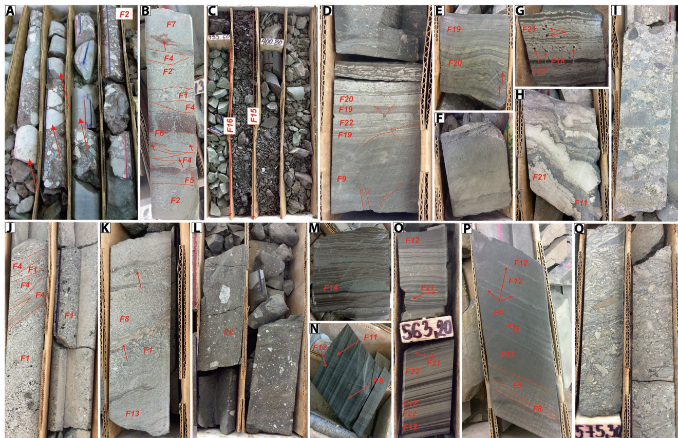
FIGURE 6 Borehole samples (width is 6 cm) represent the facies and facies associations (see code descriptions in Tables 1 and 2 ).
