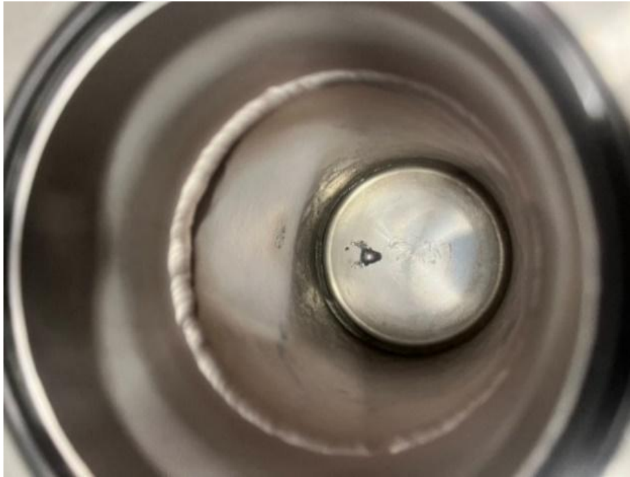
Figure 9. Photograph of sodium in the condenser after an experiment, photograph: M. Kamienowska-Orsini
