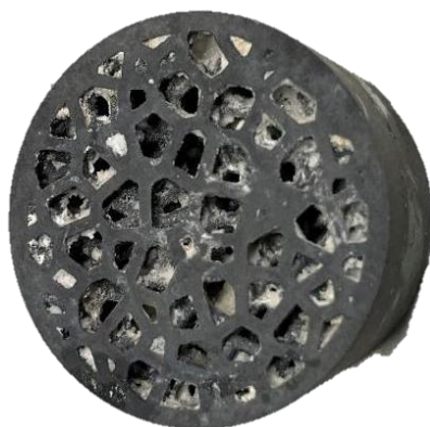
Figure 37. 3D-printed impregnated sponge, photograph: M. Kamienowska-Orsini
