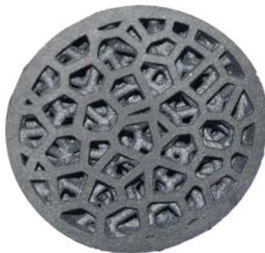
Figure 15. 20 PPI SiSiC 3D-printed sponge (OD: 38 mm), photograph: M. Kamienowska-Orsini
