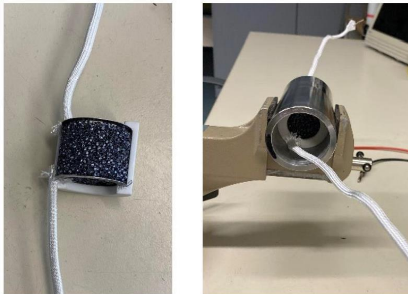
Figure 17. Images of the first concept using nickel rings instead of nickel plates, photographs: M. Kamienowska-Orsini
