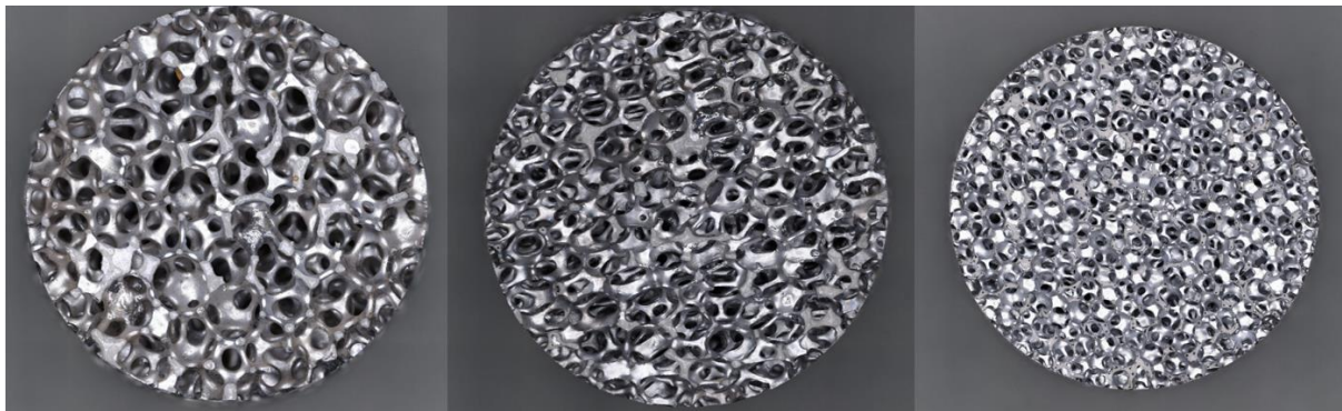
Figure 14. 10, 20 and 30 PPI SiSiC ceramic sponges (OD: 38 mm), photographs: M. Kamienowska-Orsini
