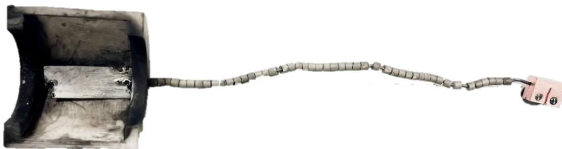
Figure 41. Macro insulation with nickel plates and wires connected to the copper adapter after the experiments, photo: M. Kamienowska-Orsini
