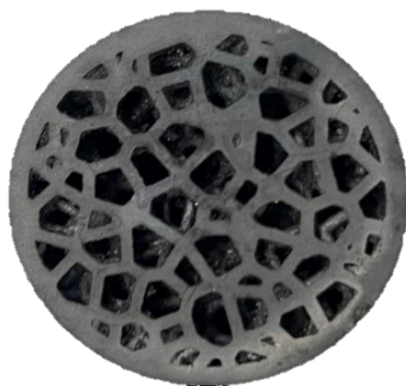
Figure 40. 3D-printed sponge after the experiments, photograph: M. Kamienowska-Orsini
