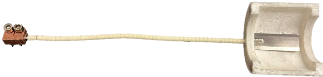
Figure 18. Macro insulation with a nickel plate and wire (with ceramic insulation beads (OD: 1.5 mm) connected to a copper adapter (photograph: M. Kamienowska-Orsini)
