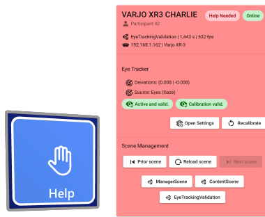
Figure 4: Pressed help button (left) and Xperisight Dashboard card (right) reflecting the state of the help button.
