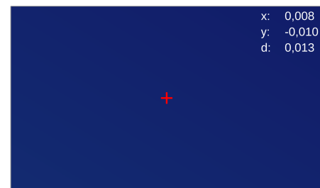
Figure 5: Unity prefab for the validation of the eye tracking calibration with optional information for debugging in the top right-hand corner.
