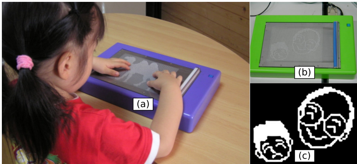
Figure A.12.: The tactile display OUV3000 from Uniplan Co. (a,b). 64x48 binary image representation (c). [70]
