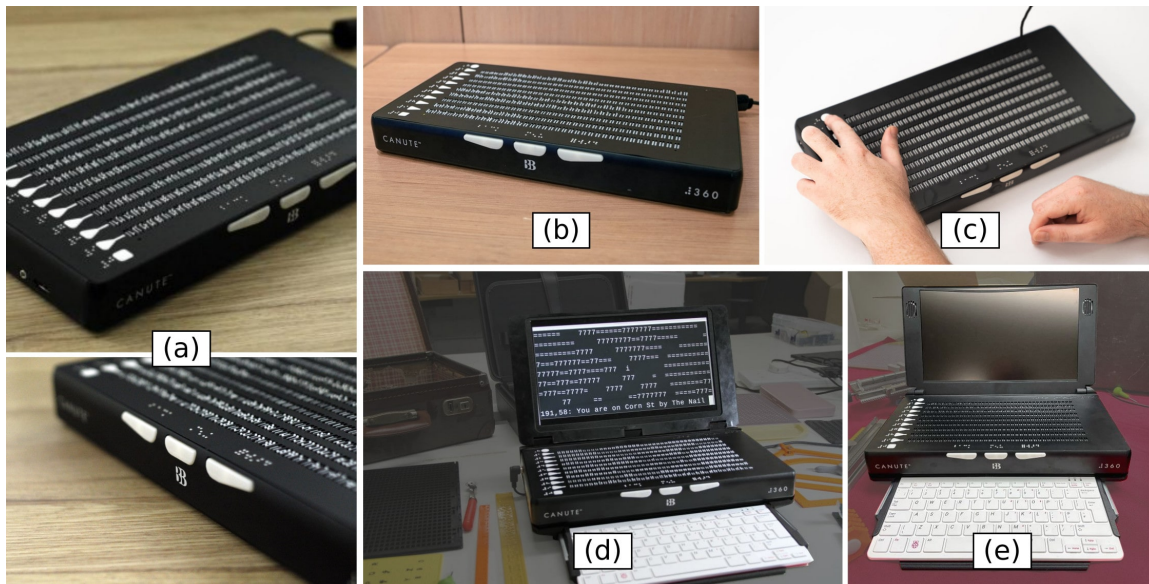
Figure A.19.: The Canute 360 standalone (a,b,c) [291]. The Canute Console (d,e) [293].
