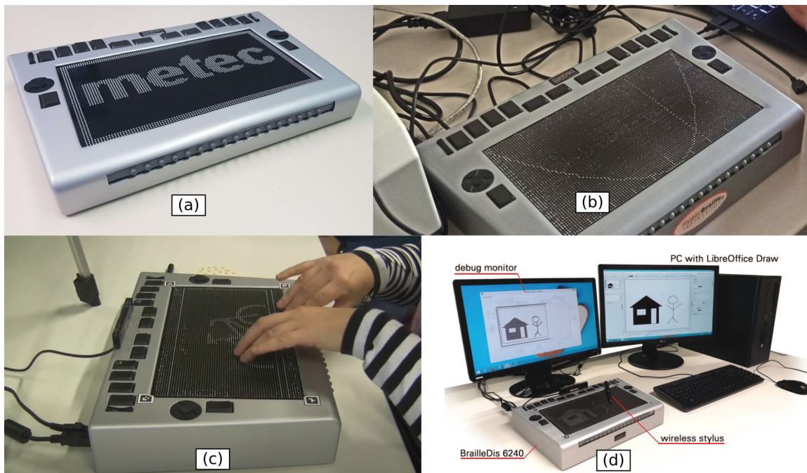
Figure A.5.: The BrailleDis 6240 (by Metec AG). (a) Pin-matrix surface with Metec icon [6]. (b) Mathematical data plots representation [265]. (c) Graphics interaction [49]. (d) Drawing workstation with wireless digitiser stylus [48].
