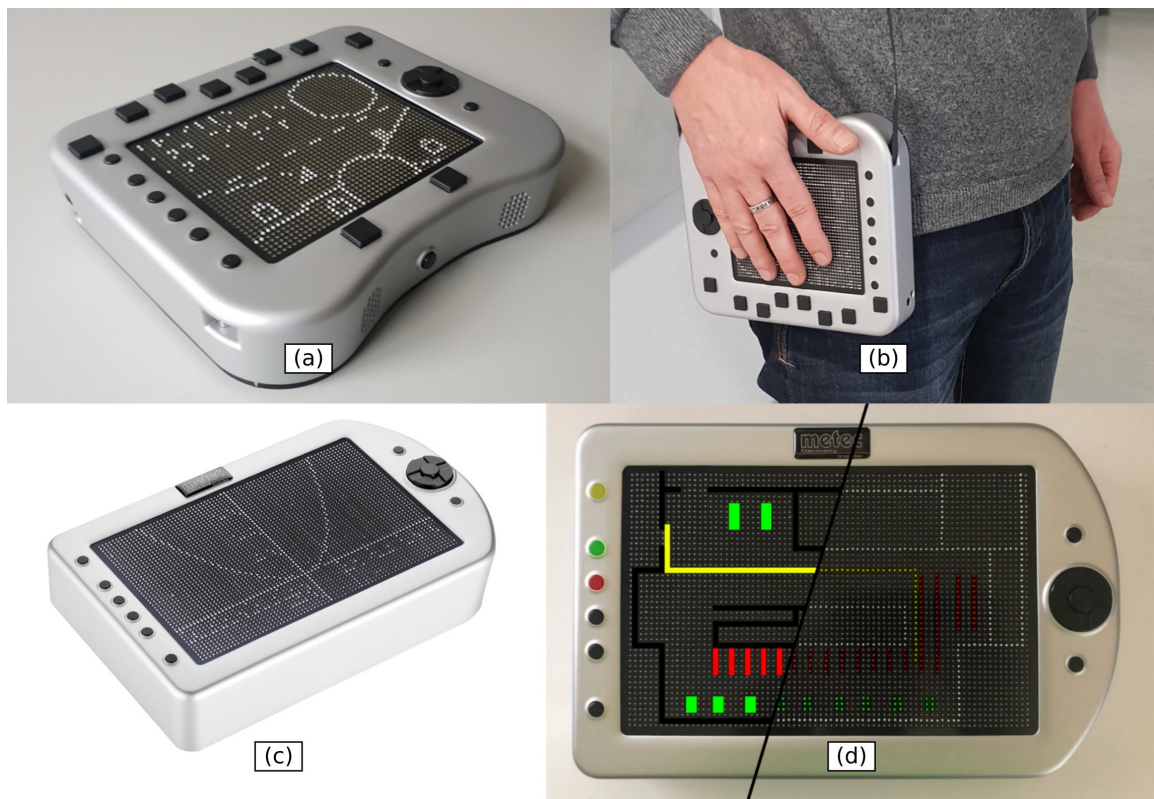
Figure A.6.: The Tactile2D and Hyperflat 2DRTP Displays from Metec AG. (a) Tactile2D with split window [9]. (b) Tactile 2D being used with a shoulder strap [45]. (c) Hyperflat representing mathematical line charts [8]. (d) Hyperflat representing floor plans [125].
