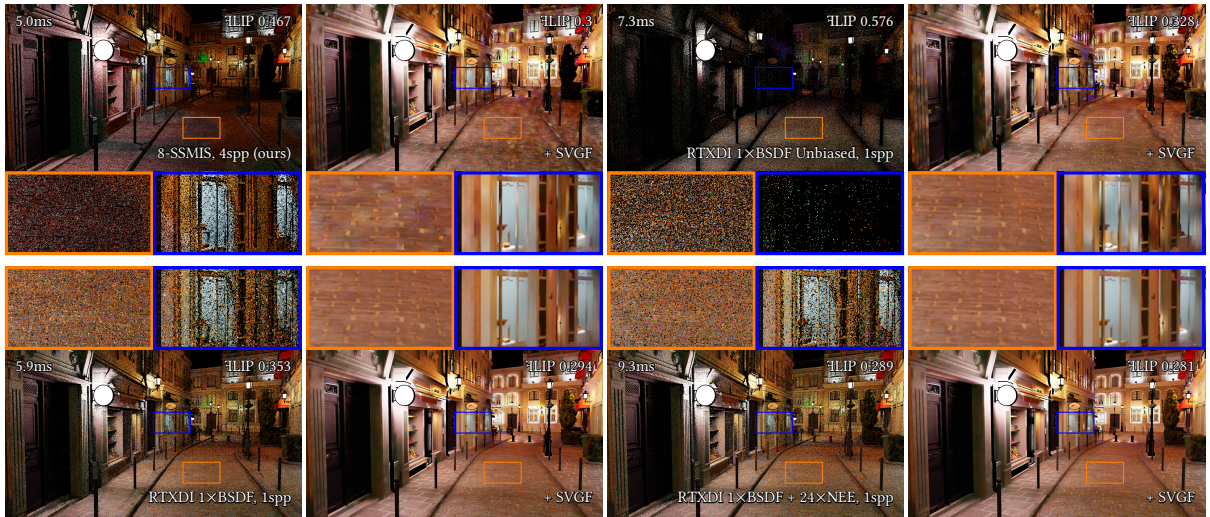
Figure 6.7.: Comparison of spatial SMIS against variants of RTXDI, a production implementation of ReSTIR [16] with and without application of a denoiser (SVGF [136]). Our approach is competitive in areas illuminated primarily by few light sources. Biased variants of ReSTIR retain image brightness better in complex regions. Figure taken from [36].
