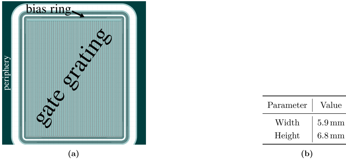
Figure 6.8.: (a) Sensor layout of a GCD test structure. All relevant parts are annotated. (b) Layout specifications of GCD capacitors.
