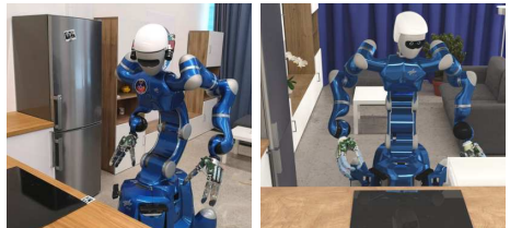
Fig. 1: DLR Rollin' Justin in kitchen scenario: real scene (left) and rendered planning map (right).
