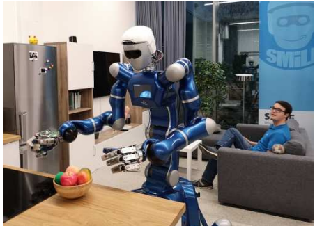
Fig. 1: Illustration of the interaction recognition problem: The robot is turned away from the operator. While the vision system might not recognize him, the audio input will do so.
