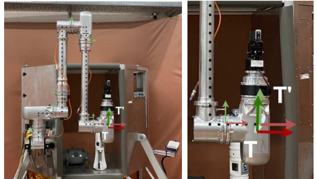
Fig. 3: TINA arm bending due to gravitation. The computed position, designated as T' , represents the theoretical location without accounting for uncertainties.
