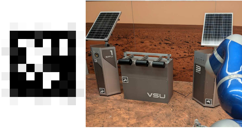
Figure 6.2.: AprilTag [145] fiducials used as visual aids for localization of objects in the environment.
