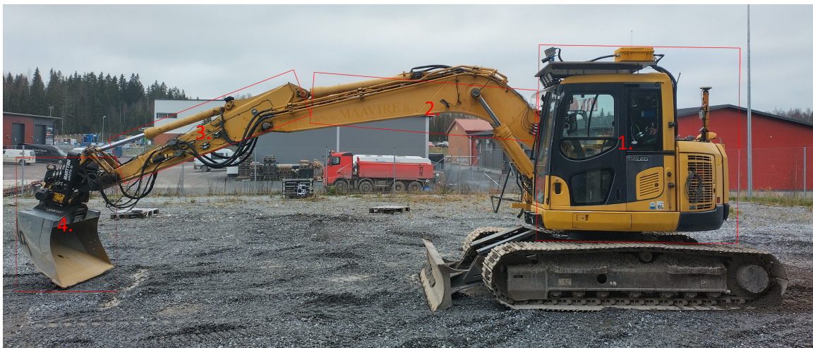
Figure 4.2: Excavator used in data collection. In the picture, (1) cabin, (2) boom, (3) arm, and (4) bucket are highlighted with red boxes [176].
