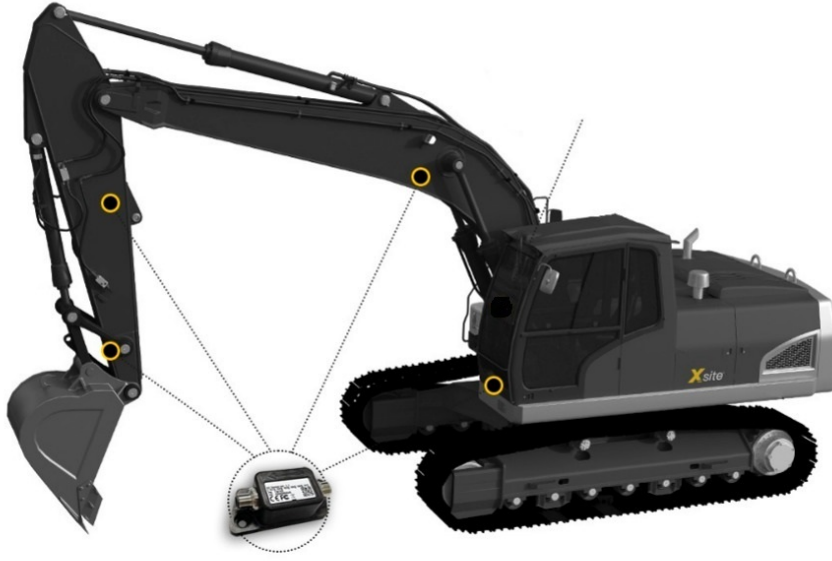
Figure 4.5: The configuration of IMUs on the excavator [177].
