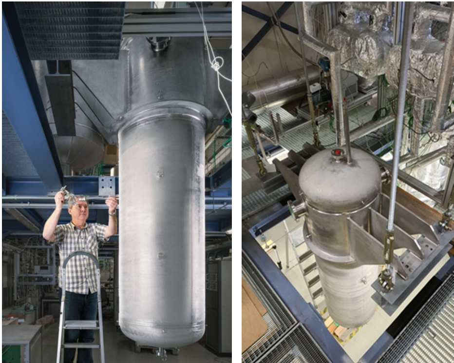
Figure 3.3: DUOLIM heat storage demonstrator during mock-up at KALLA, © by Karlsruher Institut für Technologie Campus Services – Medienproduktion (left)
