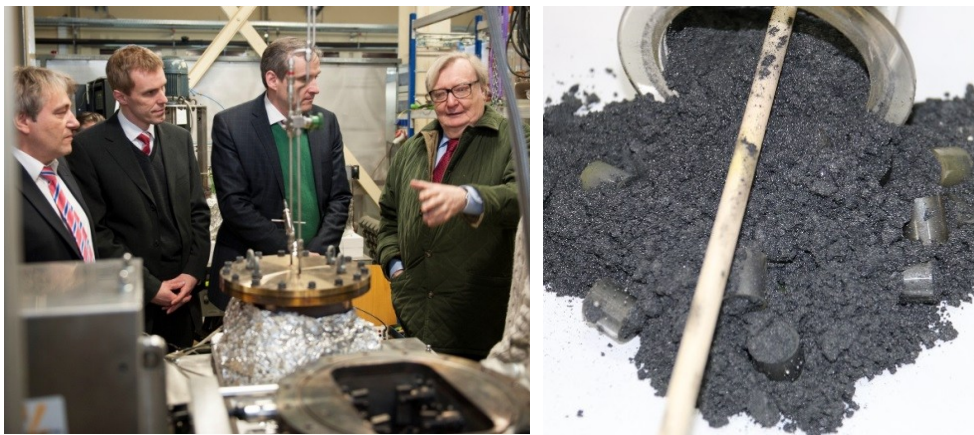
Figure 3.1: Nobel Physics Prize laureate Prof. Carlo Rubbia (right) at KIT's liquid metal material lab in 2013 and first Carbon powder produced in the HELiS plant, featuring a liquid metal bubble column.
