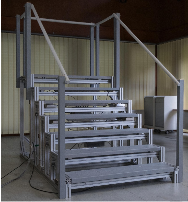
Figure 3: Picture of the instrumented staircase. Three-dimensional force plates in steps four and five from the bottom, one-dimensional force plates in steps one to three and six. Riser height = 17 cm, tread = 28 cm, inclination angle = 31.26^\circ (Steingrebe et al., 2025).
