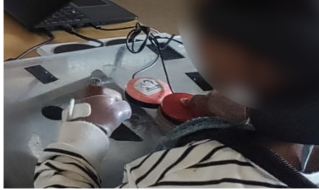
Fig. 9. Coloured buttons with stickers of different animals used for controlling forward acceleration and left and right turning of the (virtual) powered wheelchair.
