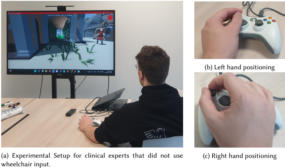
Fig. 9. a) Shows the experiment setup with clinical experts using a Xbox controller and large screen to test the game. The Xbox controller is put on the table to simulate a mounted joystick on a powered wheelchair. Depending on the preferred hand the Xbox controller was hold like b) for left handed control or like c) for right handed control.
