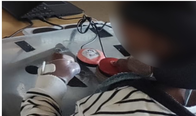
Fig. 8. Coloured buttons with stickers of different animals used for controlling forward acceleration and left and right turning of the (virtual) powered wheelchair.
