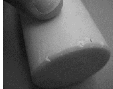
Fig. 1. Degradation of the Aluminium Oxide ceramics tube after some flashovers around 150 kV.
