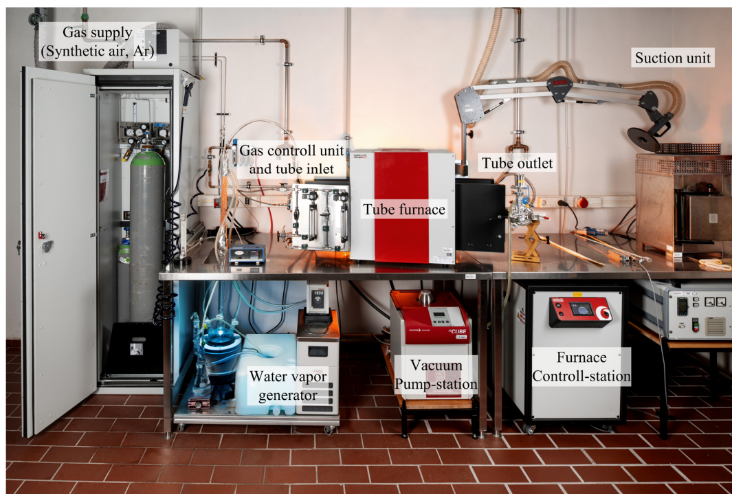
Fig. 4.7: High-temperature tube furnace for elevated temperatures, overview
