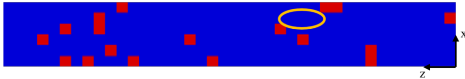
Figure 7.6: Randomly generated cohesive zone of simulation PCZ18_-60_2 with a low number of ductile element clusters near the mid thickness; initiation marked by ellipse
