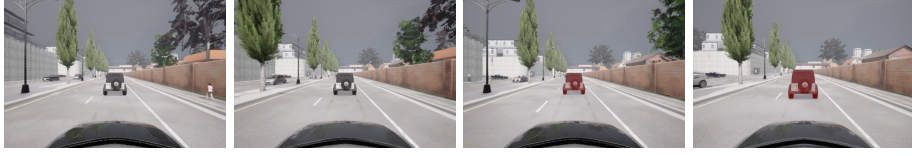
Fig. 5: Temporal anomalies: This scenario shows our implemented type of temporal anomalies. The first two images show the regular vehicle following mode. The third and fourth images show the active braking maneuver with overlaid ground truth.
