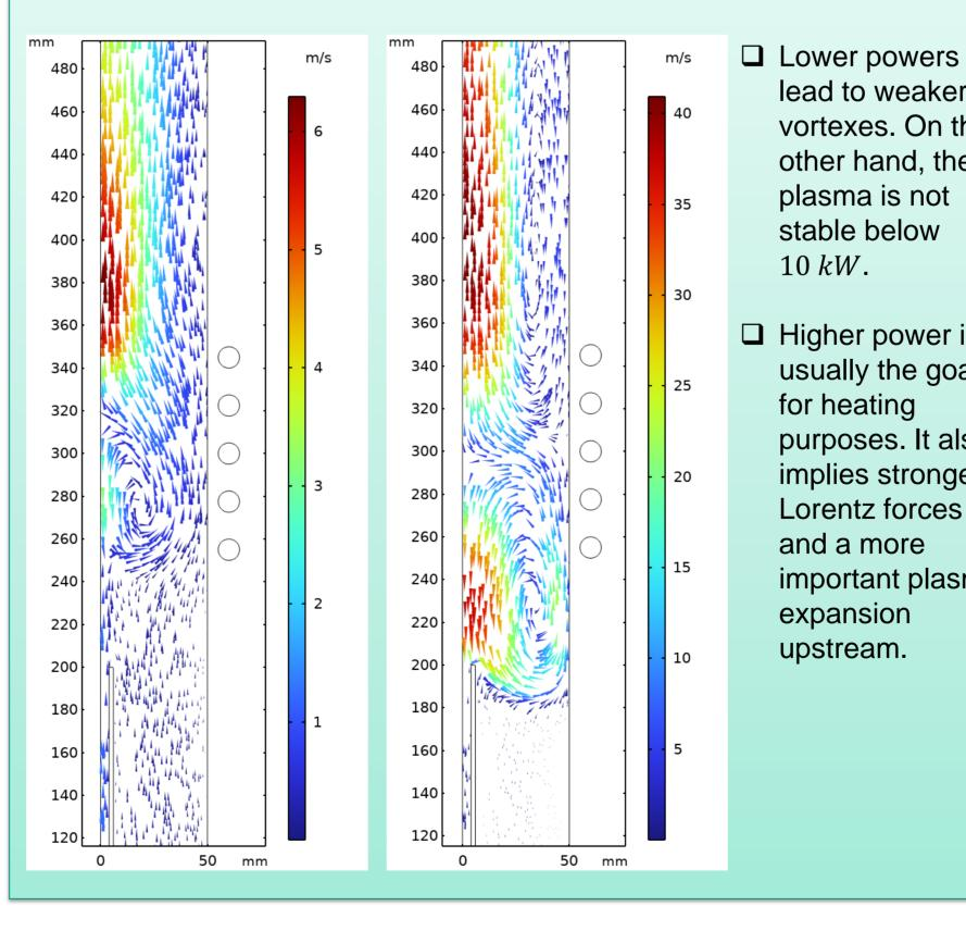
Coil power: 10 kW vs 100 kW
