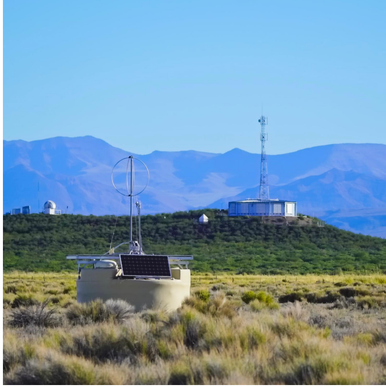
Figure 2.2: The hybrid detection of the Pierre Auger Observatory, showing a water Cherenkov detector with fluorescence detectors seen in the background.
